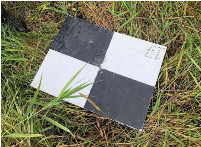
Figure 8: 1m x 1m rectangular ground control point (GCP)
