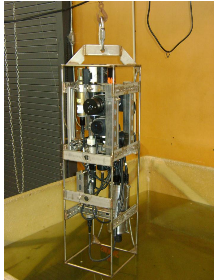
SATURN-01 instrument package undergoing final checks at the CMOP field station at MERTS, before redeployment
