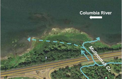
Purpose: Assess feasibility of expanding cold water plumes in the mainstem Columbia River by manipulating nearshore topography.
